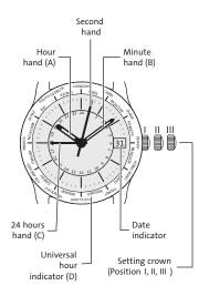
Display of local time (f. i. Reykjavik 10 p.m.) by means of hour (A) and minute (B) hand; a second time zone (f. i. New York 6 p.m.) can be selected by means of the additional hand (C), which completes one revolution in
